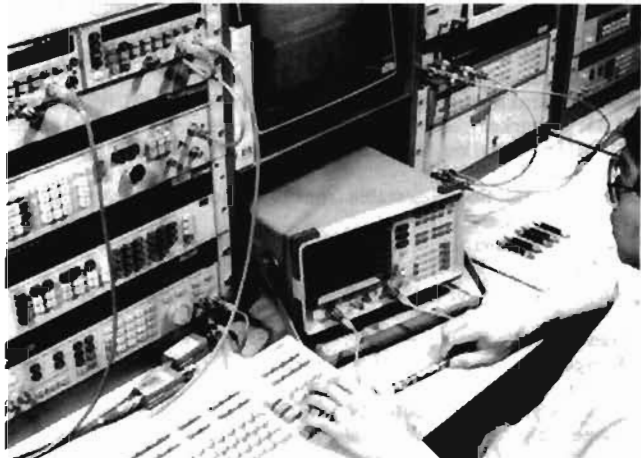
HP 8590 series RF spectrum analyzers have built-in tracking generator option
