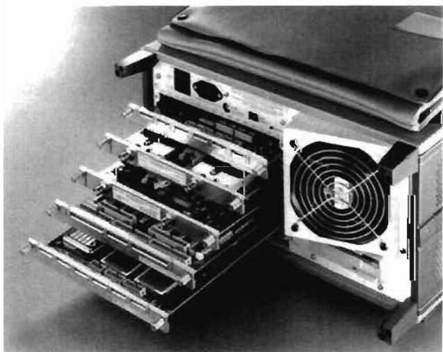
The HP 16500A supports 6 different measurement modules.
